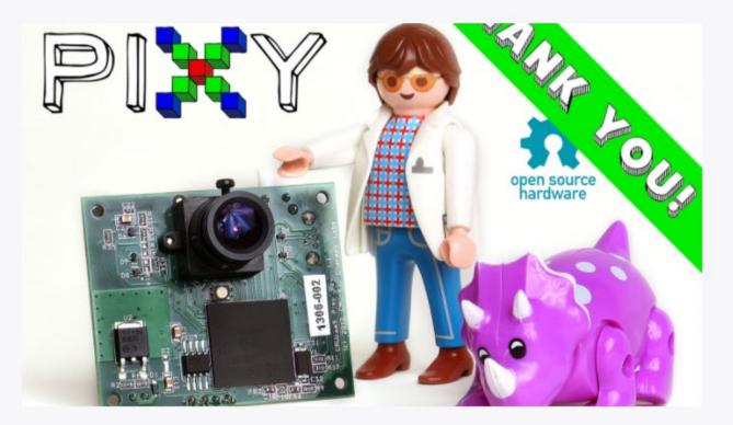
Pixy is a fast vision sensor you can quickly "teach" to find objects, and it connects directly to Arduino and other controllers.
